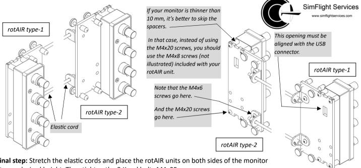
Final step: Stretch the elastic cords and place the rotAIR units on both sides of the monitor at your desired height. Then tighten the 8 Knurl bolts M4x25:
